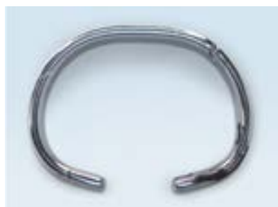
Figure 1: Abrasive wear at yarn/traveller passage
