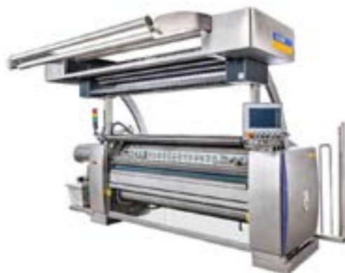
Figure 2: The new Benninger-Kusters CPB dyeing station for knitwear, the only salt-free cold dyeing process.
